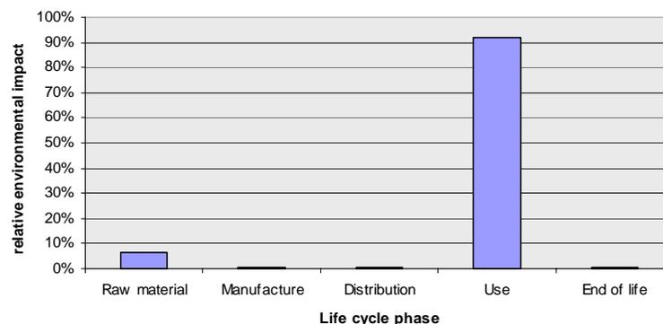
Figure 4. Step 3 - Environmental profile of the digital voice recorder [1]
